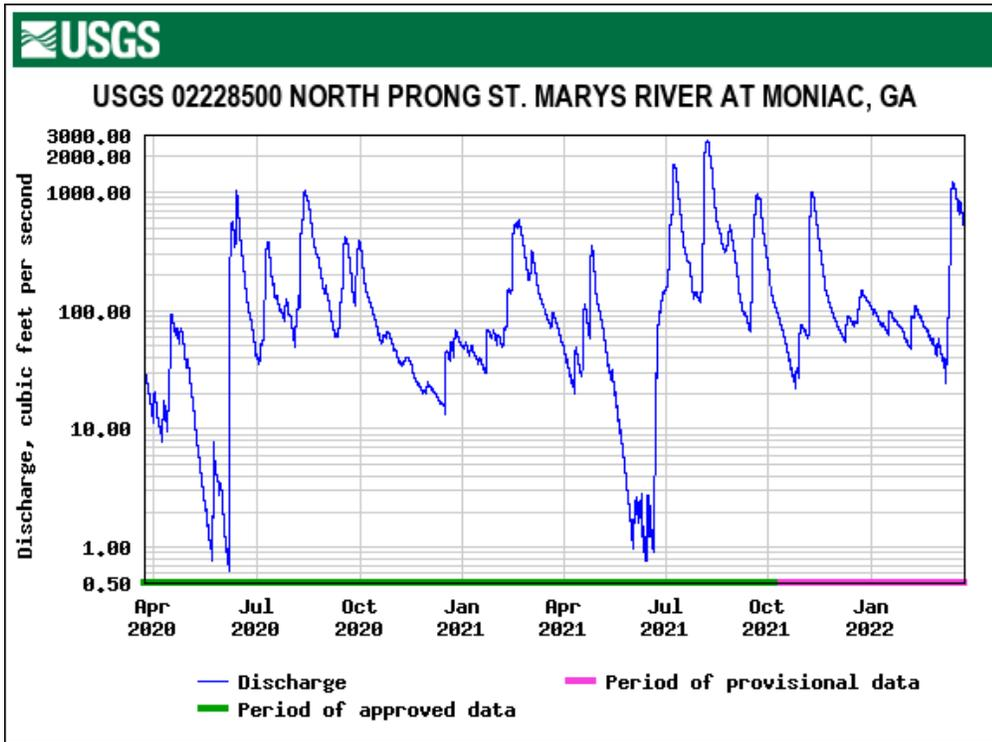
Considering the nature of flows in the upper St. Marys basin, we see that a loss of three cubic feet per second from the system could have substantial effects on the frequency and duration of extremely low flows (including zero flows) and correspondingly affect water levels in the southeastern portion of the swamp draining to the upper St Marys river.
